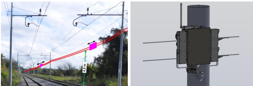
Figure 6. InspectRail concept: LiDAR sensor mounted on an autonomous mobile robot that moves along wires on the catenary poles.
