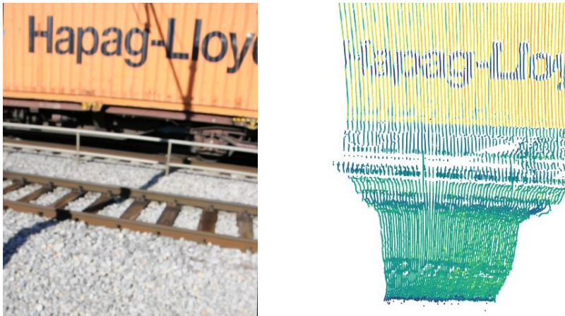
Figure 7. A container with inscription (left) and its recognition with the reflectivity measurements performed by the OS1 LiDAR sensors (right).
